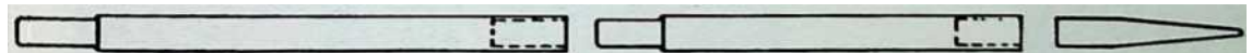
DIMENSIONS AND DISPLACEMENT DIAMETER OF TUBES.* 6'. O.A LENGTH: 22-0' PNEUMATIC VOLUME i B.CUFT. A2.3B LBS-CU.FT)' 500 LBS. DISPLACEMENT AT WATERLINE (7* DIAMj 250 WEIGHT OF SMOEL 50 LBS
